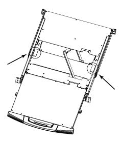
3. Attach the left and right *easy-installation* mounting rails to the inside of the rack. The flange that supports the switch will be to the inside.
